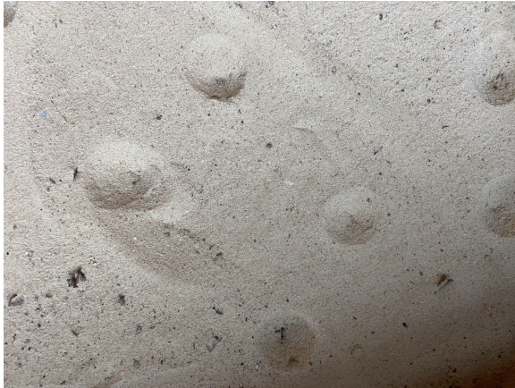
Fig 15: An image depicting the fake pits that were introduced to the 24 \times 24 trial, where a total of 12 fake pits were introduced, each with a pit depth of 5cm and a pit width of 8cm.
