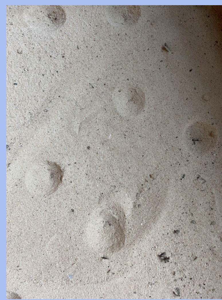
Fig 13: An image depicting the fake pits that were introduced to the 24 x 24 trial, where a total of 12 fake pits were introduced, each with a pit depth of 5cm and a pit width of 8cm.
